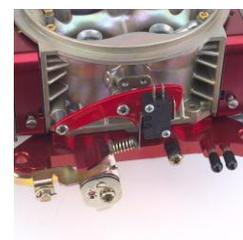
Check the switch for engagement at wide open. There should be an audible click or use a volt/ohm meter to confirm activation. If the switch doesn't activate, loosen the bracket and switch screws to realign if necessary. Also check the secondary bracket for alignment. We have supplied a couple extra idle speed screws in this package so you should be able to come up with combination that will engage the switch at wide open.
