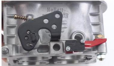
Check the switch for engagement at wide open. There should be an audible click or use a volt/ohm meter to confirm activation. If the switch doesn't activate, the left hole of the micro switch is slotted to realign if necessary.
