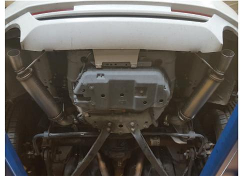
7. Place (x2) **black tips (3)** onto mufflers and tighten inlets. Rotate components to desired distance from body or bumper, so angle cut on tips are properly positioned.
