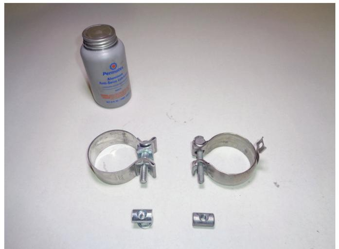
6. Place (x2) ball clamps (removed step 4) onto **left (1)** and **right (2) mufflers** then install them onto vehicle, inserting wires into isolators. Tighten clamps just enough for later adjustment.
