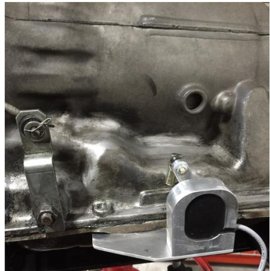
Sensor Mounted on a Turbo 350 Transmission
