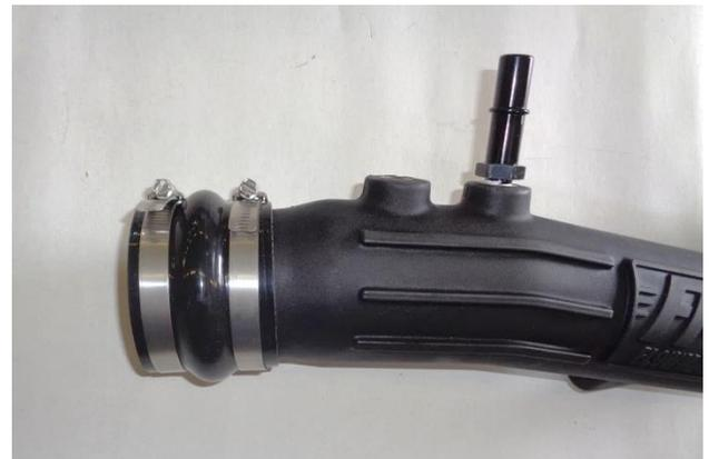
23. Install two small hose clamps (16) on small flex coupler (17), and install coupler on discharge end of intake tube. Only snug the clamps at this time, to allow adjustment when tube is installed.
