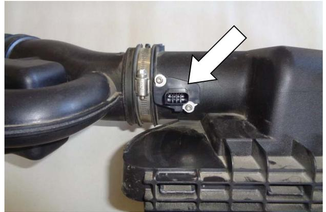
11. Remove the MAF sensor from the airbox, then remove the stock gasket from the sensor.
