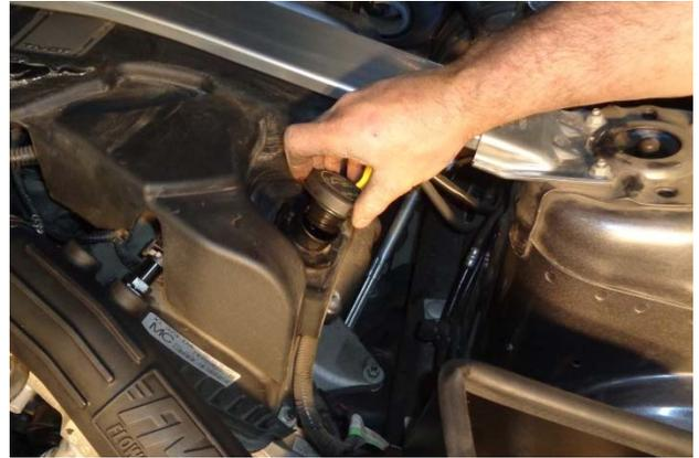
34. If your vehicle includes the optional engine cover, remove the oil fill cap, reinstall the fill cap extension (removed at Step 4), then reinstall the fill cap.
