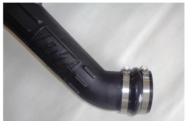
24. Install two large hose clamps (21) on large flex coupler (12), and install coupler on intake end of intake tube. Only snug the clamps at this time, to allow adjustment when tube is installed.
