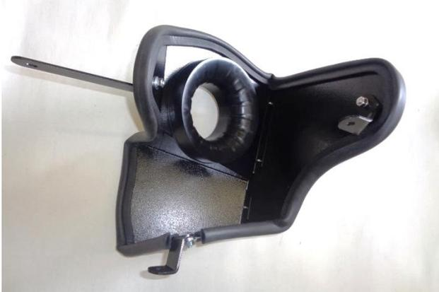
19. Attach the gasket (24) to the heat shield. Starting on either side of bracket (8), gradually work around the heat shield, firmly pressing the seal onto the edge. When you return to the bracket, trim seal to fit using metal-cutting shears.
