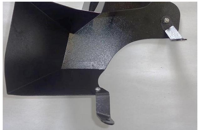
17. Attach bracket (8) to heat shield using  $\frac{1}{4}$ -20  $\times$   $\frac{5}{8}$ " screw (9) (against bracket), and flat washer (7), lock washer (5) and nut (6) (against heat shield).
