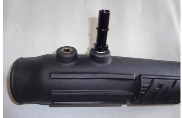
22. Your vehicle may require one or both vacuum fittings. If it uses only one fitting, the 1/4" plug (20) will be used in the unused port. Apply 2 wraps of nylon thread tape to threads of the required hardware, and install them in intake tube (15), in the appropriate ports.
