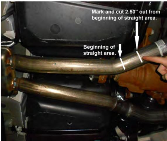
2) Begin by measuring back 2-1/2" from the beginning of the straight area shown in the photo at left and make a mark on both pipes. Support the exhaust system both in front and behind the area to be cut. Check that the marks are correct, then using a reciprocating saw, cut both pipes at the marks. **Note: Due to the closeness of the pipes to the gas tank, use caution when cutting!** Carefully deburr the end of the muffler inlet pipes where cut with a file or die grinder.
