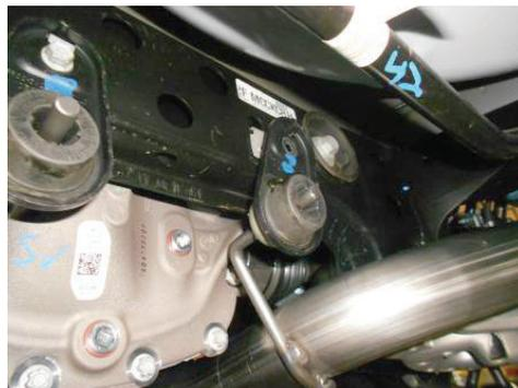
10. Adjust and level mufflers for a satisfactory fit. Maintain a minimum of ½" clearance around all components of exhaust system, keeping in mind suspension, travel and vibration. After making any required adjustments, securely tighten all clamps.
